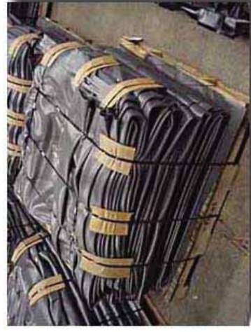
Prefabricated liner ready for dispatch
